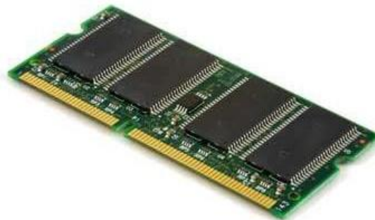
Figure 6.24 – Printed circuit board containing computer memory
