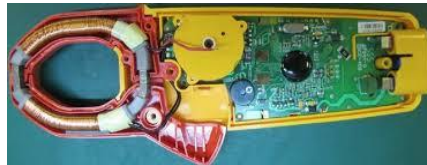
Figure 5.1 – Sectional View of an AC Clamp Meter
