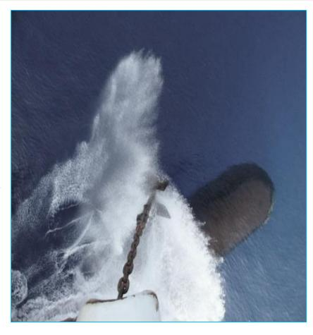
During all manoeuvring and harbour operations, one team is always assigned to anchor operation for emergency stop of the ship (during engine or steering failure).
