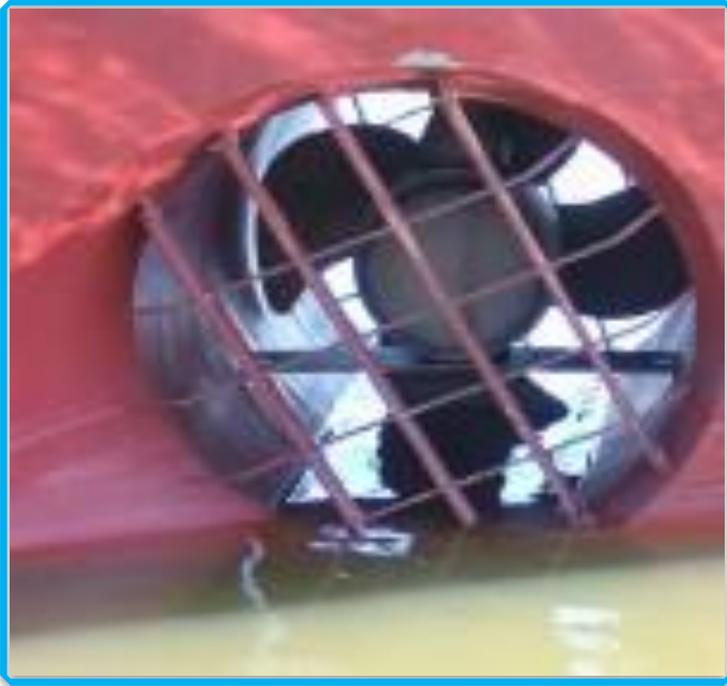
“Thrusters are type of propellers, smaller in size, which help in better manoeuvrability of the ships at lower speeds.”
