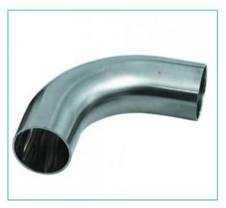
In a long radius elbow the radius of curvature is 1.5 times the nominal diameter. In a standard elbow the radius of curvature is 1.0 times the nominal diameter of the pipe.
