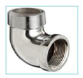
A street elbow is different from the male and female elbows in the respect that it has a male thread on one side and a female thread on other side. The advantage of using the street elbow is that it can directly fix to the pipe without connecting a nipple. They come in various angles like 45 degrees and 90 degrees.
