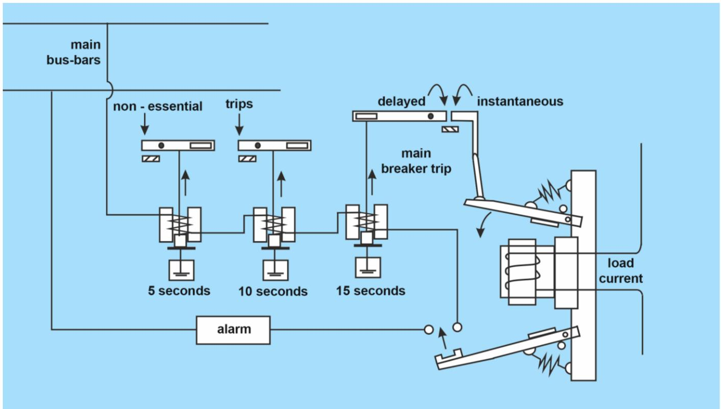
The current passes through the electromagnetic coil and the linkages are kept from contacting using a spring arrangement. As soon as the current value increases the limit, the electromagnetic coil pulls the linkage up against the spring force and operates the instantaneous circuit and the alarm system. The lower linkage completes the circuit for the preferential trip circuit.
