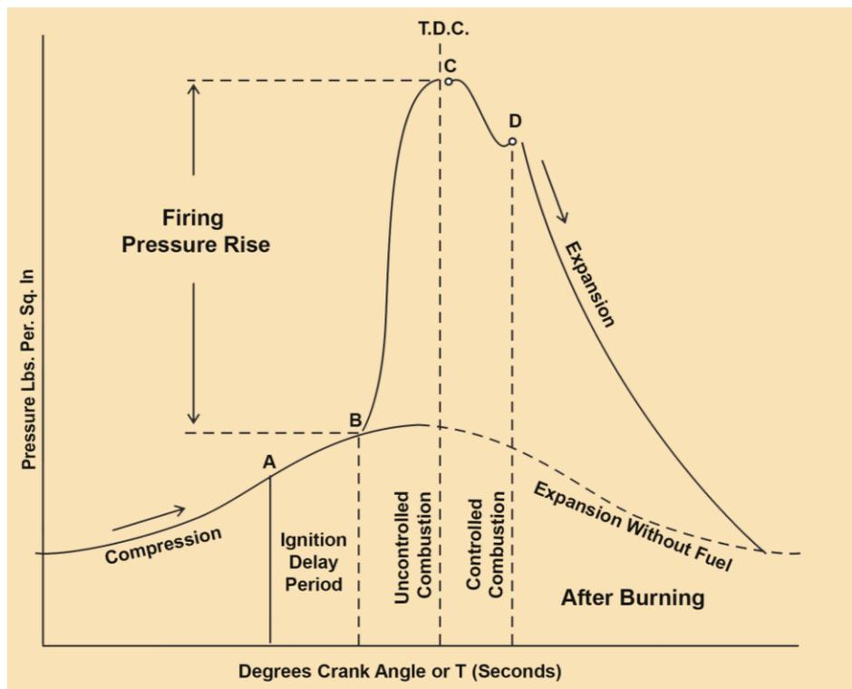
From the graphs obtained, various characteristics such as engine timing, compression pressure, cylinder output etc. can be analyzed.
