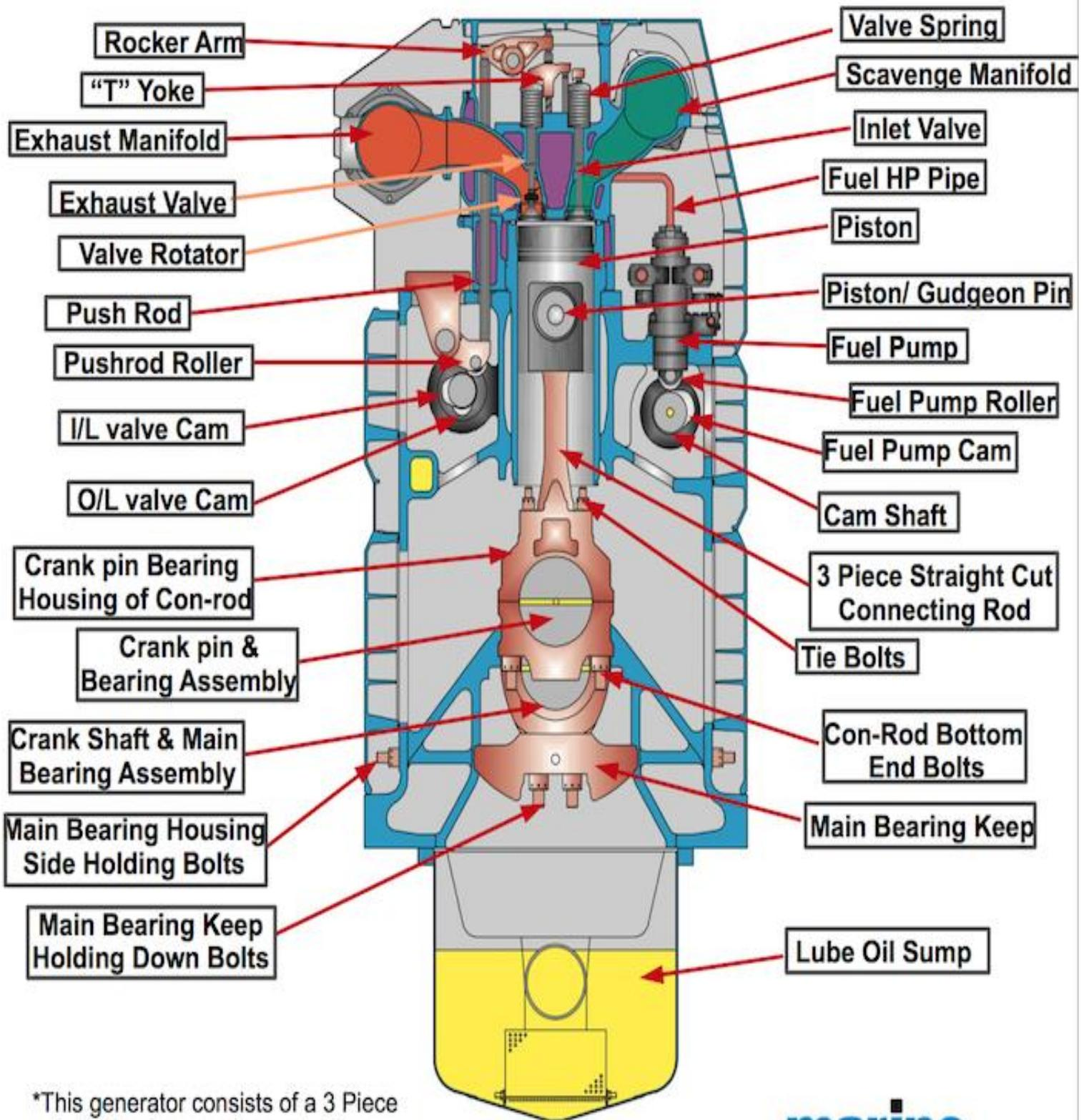
\*This generator consists of a 3 Piece straight cut connecting rod with an underslung crankshaft
